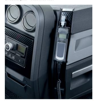
74 23 253 861 Breathalyser - Alcolock test, left-hand drive 74 23 253 862 Breathalyser - Alcolock test, right-hand drive
