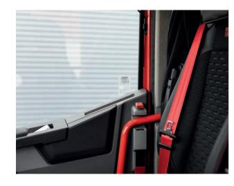
Mechanical anti-intrusion Doorlock
